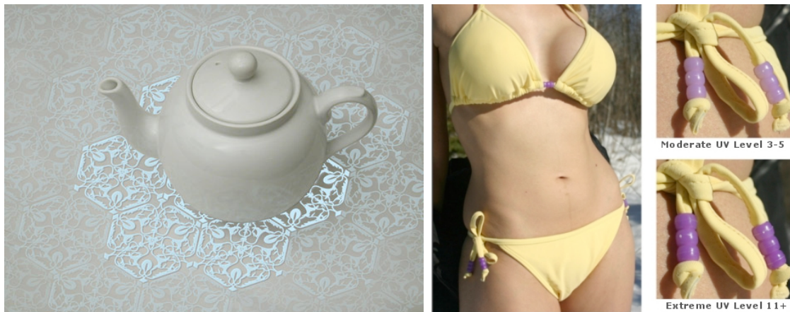
Figure 3: The History Tablecloth 2 (left) has a pattern of embedded electroluminescent material that begins to glow when objects are placed upon the surface. When objects are removed the pattern begins to fade slowly. The SmartSwim UV Intensity Bikini 3 (right) uses UV sensitive materials to warn against excessive exposure to the sun.
