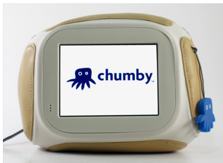
Figure 2. Chumby has an accelerometer, a touchscreen and uses Wi-fi to connect to the Internet.
