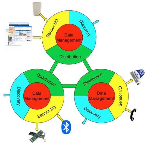
Figure 1. Data from sensors like Bluetooth or RFID is aggregated by nodes, which then disseminate the information.
