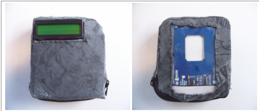
Figure 3.1: System Form Factor: Left image shows the front of the pouch with an integrated LCD display. Right image shows the back of the pouch with RFID reader.
