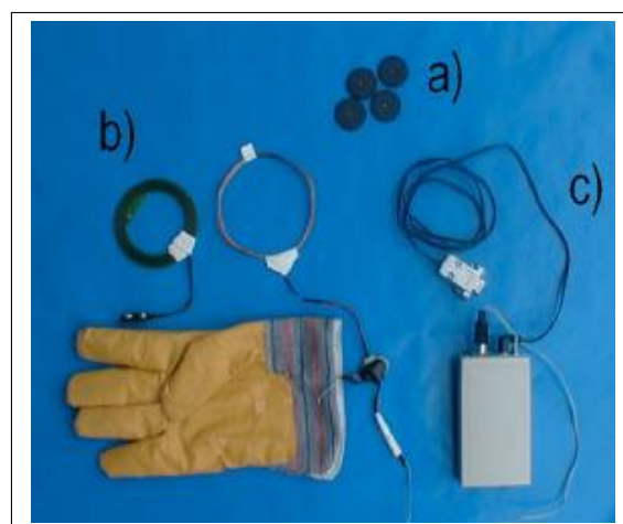
Figure 2.3: RFID glove components (from Schmidt and Gellerson [10]): a) RFID Tags, b) Reader Coils, c) Wearable Tag Reader
