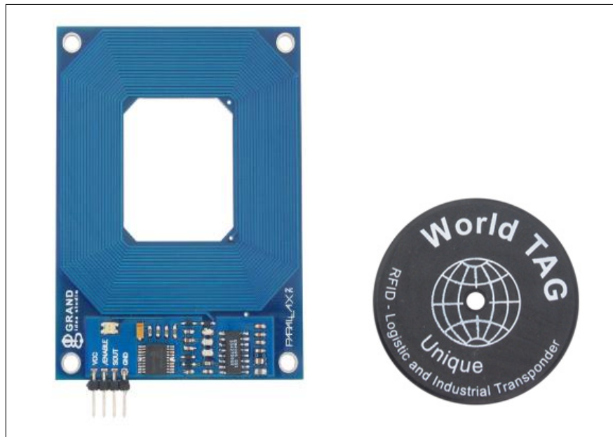
Figure 2.1: Left) RFID reader used in ReFInDer: measures 62.22mm x 82.5mm, Right) Example RFID tag: measures 50mm in diameter [14]
