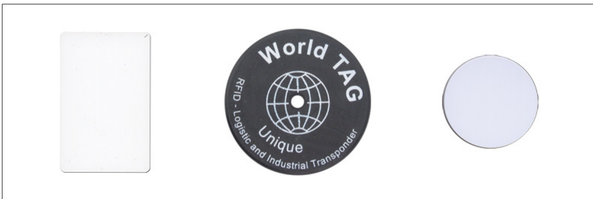
Figure 4.2: RFID Tags: Left) Rectangular Tag, Center) Circular Tag (50mm), Left) Circular Tag (25mm) [14]
